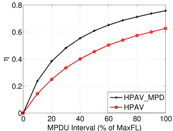
Fig. 5. MAC Efficiency as a function of MPDU Interval.
