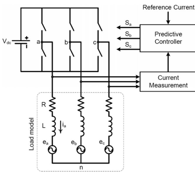
$$\mathbf{v} = \frac{2}{3} (v_{an} + \eta v_{bn} + \eta^2 v_{cn}), \quad \eta := e^{j2\pi/3}$$
