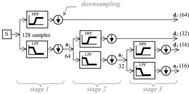
Fig. 1. 3-level DWT
