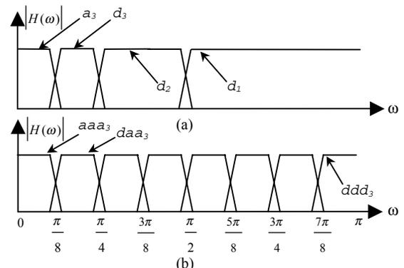
Fig. 3. Frequency bands for the analysis tree
