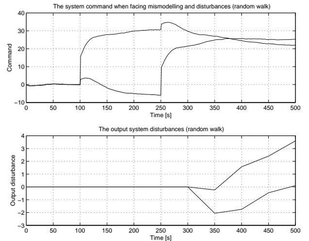
Figure 6: The disturbance profile across the batch together with the command moves
