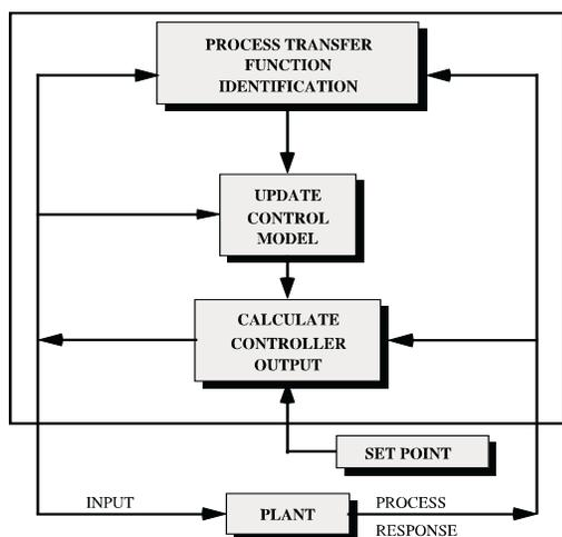
Figure 3: The closed loop of the advanced control system applied to the batch reactor
