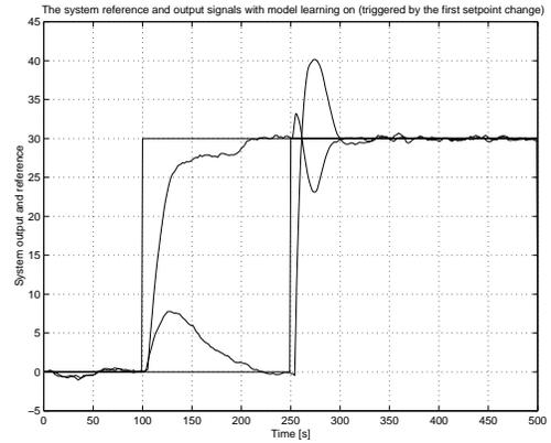
Figure 5: Time responses for a sequence of steps in the reference signals subject to random walk type of disturbances
