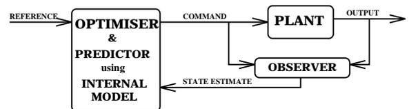
Figure 2: The structure of *MBPC* schemes
