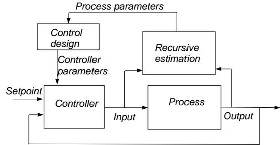
Figure 2: Indirect self-tuning control
