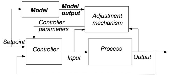
Figure 1: Model-reference adaptive control
