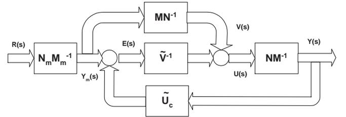
**Figure 7:** Coprime Factor Formulation of Self Tuners (Model Following Equivalent)
