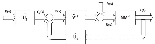
**Figure 6:** Coprime Factor Formulation of Self Tuners
