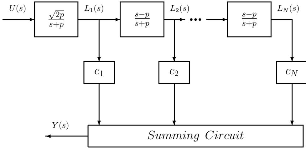
**Figure 4:** Representation of plant dynamics using a truncated continuous Laguerre ladder network.
