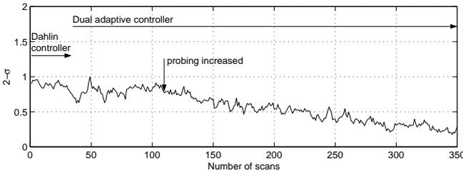
**Figure 5:** Trial 3, the benefit of probing is illustrated. From top: profile  $2\sigma$ ; some gain estimate profiles; some actuator profiles; some CD coat weight profiles
