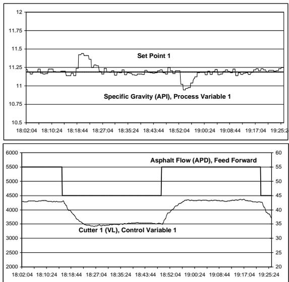
Fig. 3. The closed loop control of specific gravity tests, model identification and control optimization took three days.
