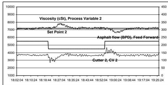
Fig. 4. The closed loop control of fuel viscosity
