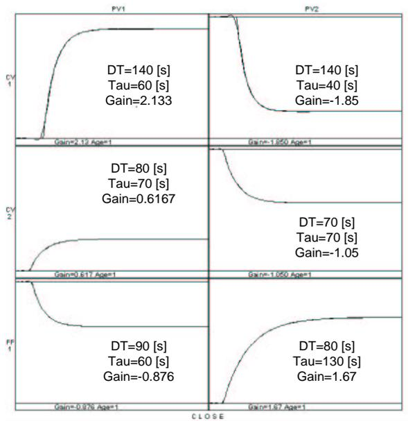
Fig. 2. The plant and feedforward models
