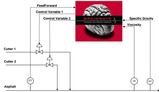
Fig. 1. The closed loop with the advanced adaptive MIMO controller
