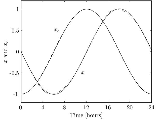
**Figure 2:** Unforced response ( $I=0$ ) of  $x$  and  $x_c$  with linear approximation ( $\mu=0$ ) of equation (1) (solid line) versus the original nonlinear form (dashed line).
