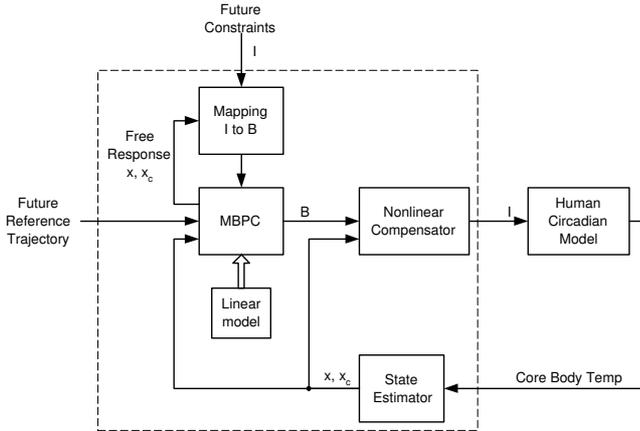
**Figure 3:** Controller architecture.
