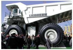
Liebherr T282B earthhauling truck 2.7MW AC Propulsion
