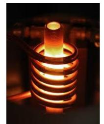
No Flame Heater for Dental Instrument
