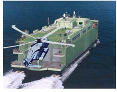
Future Canadian Ship: Joint Support Ship (JSS) 30.4MW Electric Propulsion
