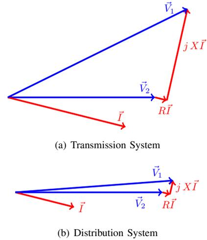
Fig. 4. Phasor diagram of voltages in a two-bus system for a typical transmission and distribution line.
