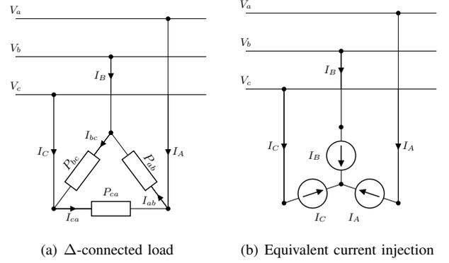
Fig. 1. A  $\Delta$ -connected load and its equivalent Y-connected current injection.
