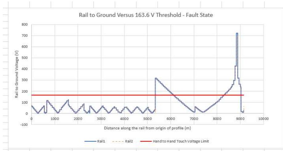
Figure 8 – Case Study 2: Rail to ground voltage during fault state with locomotive shunting a pair of insulating joints.
