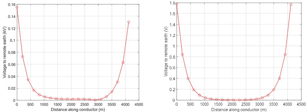
Figure 5 – Case Study 1: Typical induced voltage on a continuous earthed fence under fault (left) and in steady-state (right)
