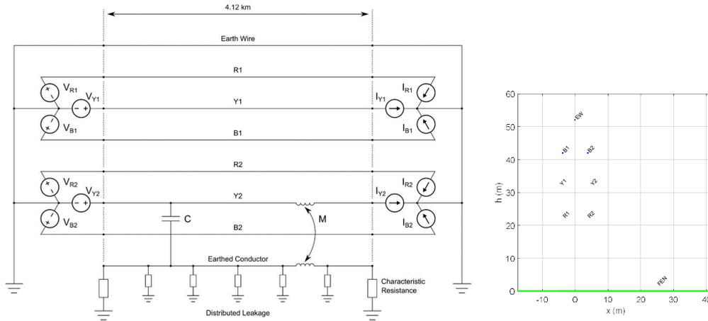
Figure 4 – Case Study 1: MTL model for NG 400 kV line interface with a HS2 conductor
