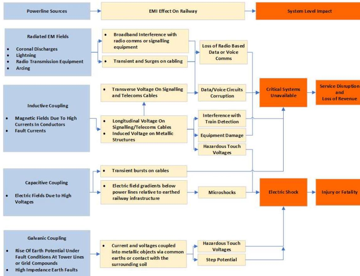
Figure 2 – Powerline sources of interference and impacts on railway systems.
