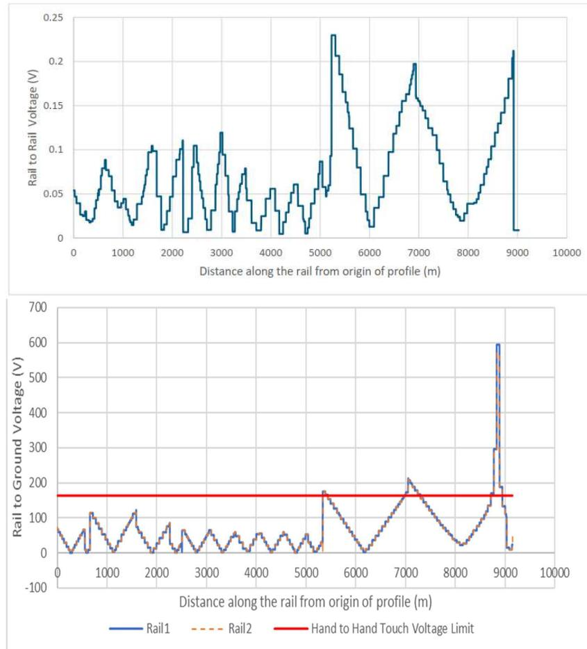
Figure 7 – Case Study 2: Rail to rail voltage during steady state (top) and rail to ground voltage in fault-state (bottom) power line operation.
