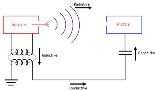
Figure 1 – Coupling mechanisms between powerlines and nearby metallic objects.
