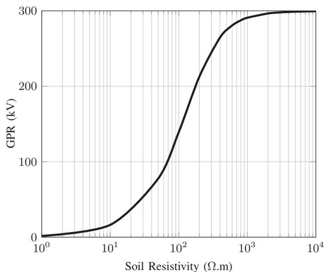
Fig. 4. Tower ground potential rise as a function of local soil resistivity (pre-fault voltage 1.04 pu).
