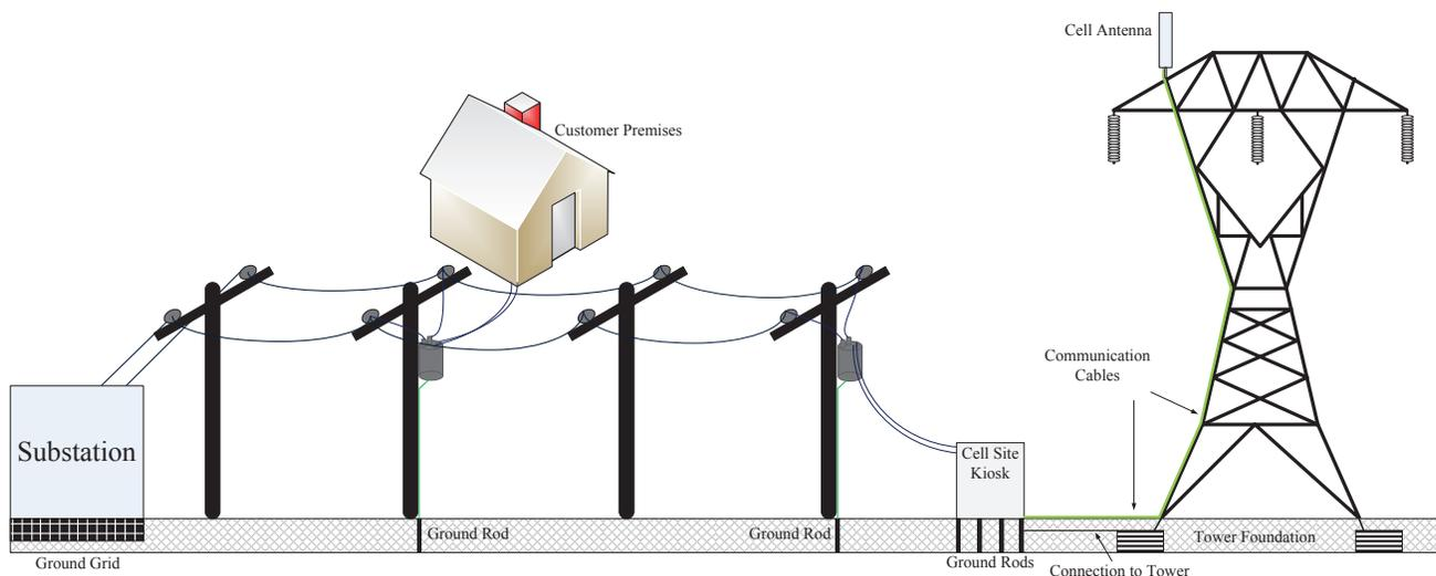
Fig. 1. Typical LV power supply scheme to a cell site compound installed next to a transmission tower.
