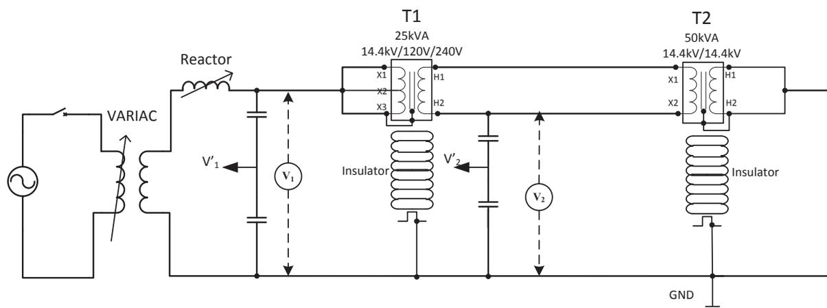
Fig. 7. Equivalent circuit of the voltage withstand test at a high-voltage lab using a resonant test system.
