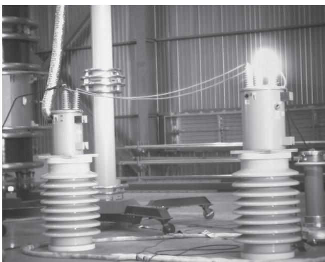
Fig. 8. Voltage withstand test at a high-voltage lab using a resonant test system. The left hand-side transformer is a 14.4 kV/120 V, 25 kVA service transformer, the right hand-side transformer is a 14.4 kV/14.4 kV, 50 kVA isolation transformer. The external flashover across the bushings of the isolation transformer is visible (at 125 kV-RMS).
