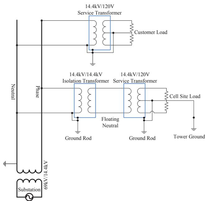
Fig. 6. Proposed LV supply circuit to minimize the risk of GPR transfer from HV system to LV system.
