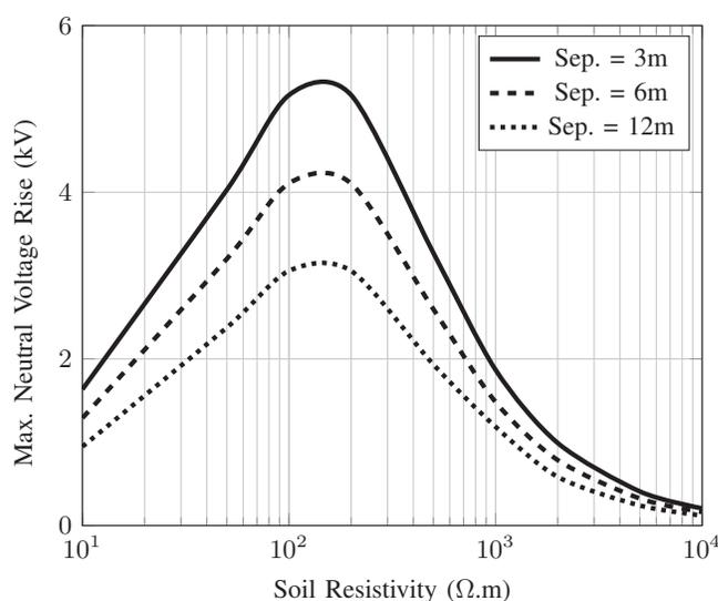
Fig. 9. Maximum voltage rise on the distribution neutral transferred through the soil to the isolation transformer ground rod (connected to the multi-grounded neutral) for various separation distances between the isolation and service transformers poles (5 km to the substation, station grid resistance = 0.5 Ω).
