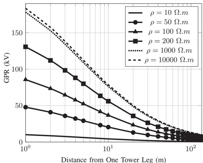
Fig. 10. GPR profiles calculated at various distances from one tower leg for various soil resistivity conditions.
