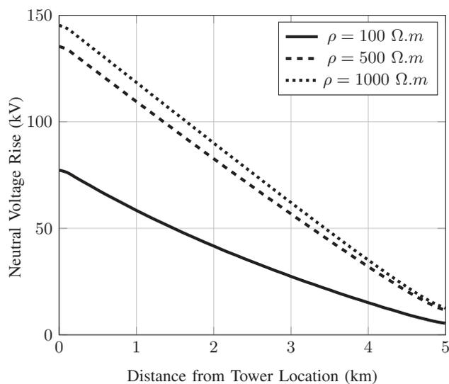
Fig. 5. Voltage profile along the distribution neutral bonded to the transmission tower for various soil resistivity values (5 km to the substation, station grid resistance = 0.5  $\Omega$ ).
