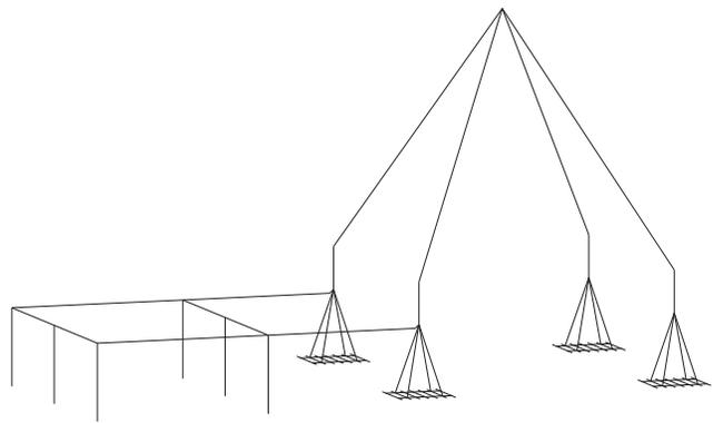
Fig. 3. Typical tower foundation (rigid-tower, grillage foundation), cell site compound ground grid (ground rods and counterpoise wires), and relevant connection between the two.
