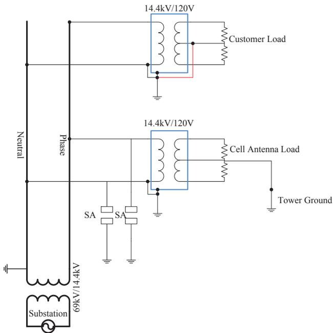
Fig. 2. Historical isolation method used to minimize the risk of GPR transfer from HV to LV system.
