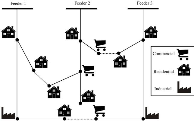
Figure 7. The 14-node test system with hypothetical load composition.
