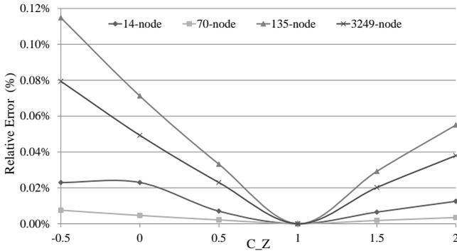
Figure 4. Average relative errors between nodal voltages obtained by the LPF method and the implicit Z-bus method (obtained by (21)) as a function of  $C_Z$ .
