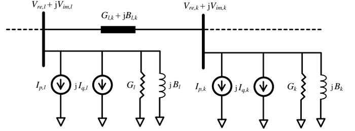
Figure 2. Generic part of a DS obtained based on the LPF load synthesis.
