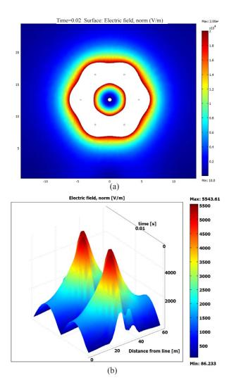
Fig. 5: Electric field intensity for circular-type 230kV 3-circuited according to Fig. 2b right side arrangement at t= 2ms (a) and for time versus distance from the TL (b)
