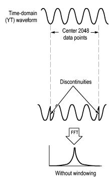
Applying a window to the YT waveform changes the waveform so that the start and stop values are close to each other, reducing the discontinuities.
