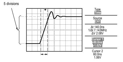
**NOTE**. The Rise Time measurement is available as an automatic measurement in the Measure Menu. (See page 89, Taking Measurements.)
