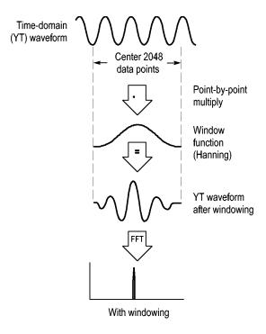
The Math FFT function includes three FFT Window options. There is a trade-off between frequency resolution and amplitude accuracy with each type of window. What you want to measure and your source signal characteristics will help you to determine which window to use.
