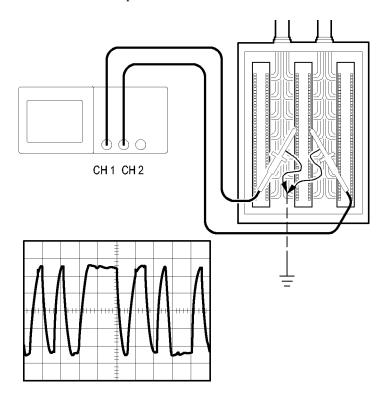
**NOTE.** Be sure to first compensate both probes. Differences in probe compensation appear as errors in the differential signal.
