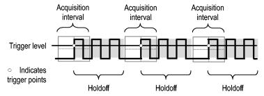
Triggers are not recognized during holdoff time.
