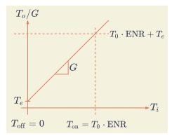
The noise source outputs a noise level defined by its "excess noise ratio" (ENR) =  $T_{\rm on}/T_0$ . Since the noise source and amplifier-generated noise are independent, their powers will add and it's possible to solve for  $T_e$  and F.
