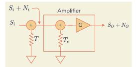
The amplifier outputs a signal power  $S_o = GS_i$ . If the noise input power is  $N_i = kTB$  then the noise output power is  $N_o = Gk(T + T_e)B$ . The noise figure is thus:
