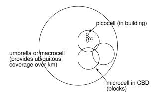
To allow for ubiquitous service as well as high user density, cells of different sizes are overlaid. The larger "umbrella" cells provide ubiquitous coverage while the smaller cells provide capacity in areas with high user density.
