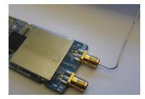
You may want to run the LimeSuite utility from the Windows Menu to verify the connection to the SDR board. Select Options/Connection Settings, select the LimeSDR Mini device, and click on connect. If you now click on the buttons Defaults and Calibrate All, the device will take a few seconds to calibrate itself and then show new DC and gain offsets. This verifies the board is connected and functional.
