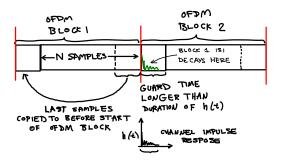
Since no (new) data is transmitted during the guard time, this reduces the average data rate. However, the guard time is typically a small fraction of the OFDM symbol duration and so the impact on the overall throughput is relatively small.
