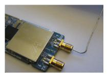
You may want to run the LimeSuite utility from the Windows Menu to verify the connection to the SDR board. Select Options/Connection Settings, select the LimeSDR Mini device, and click on connect. If you now click on the buttons Defaults and Calibrate All, the device will take a few seconds to calibrate itself and then show new DC and gain offsets. This verifies the board is connected and functional.
