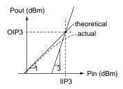
The power at which the third-order component would have the same power as the fundamental is called the third order intercept point (IP3). This can be an input power (IIP3) or output power (OIP3). The two are related by the theoretical gain of the amplifier.
