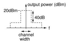
You may assume that the adjacent-channel power is caused solely by third-order intermodulation products. Thus, the power of any intermodulation products falling in the adjacent channel must be 40 dB below the power of the in-channel signals.
