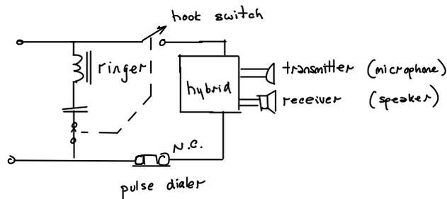
When the phone is on-hook the ringer is connected across the line through a capacitor. Thus the phone appears as an open circuit at DC but AC current can flow through the ringer to ring the phone.
