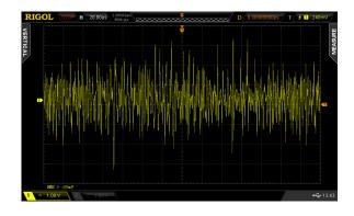
Enable the (MATH) trace showing the FFT operation to view the spectrum of the signal. Set the vertical scale to 5 dB/division. Adjust the Horizontal scale to show a frequency range covering the ADSL signal bandwidth.
