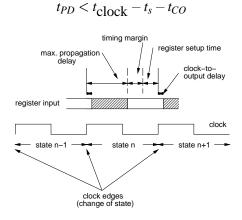
Using a single clock means we only need to compute the delay through *combinational* logic blocks which is much simpler than having to predict the effect of propagation delays on clock signals. This is why almost all large-scale digital circuits are synchronous designs.
