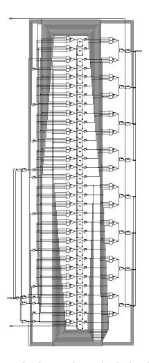
For many implementation technologies (FPGAs, gate arrays, or standard-cell ASICs) there are usually vendor-specific ways of implementing memory arrays that give better results. However, using a VHDL-only model with "random logic" as shown above is more portable and may be practical for small memories such as CPU "register files."
