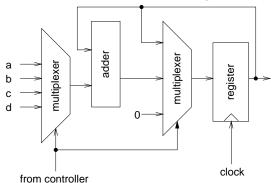
**Exercise 45**: Other datapaths could compute the same result. Draw the block diagram of a datapath capable of computing the sum of the four numbers in three clock cycles.
