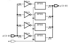
Tri-state outputs are used primarily to implement bidirectional bus signals. Bidirectional buses are declared of type inout rather than in or out and their values can be both 'read' and 'written' within the architecture (unlike signals of type out). When the bus is to act as an input, the bidirectional bus signals are driven to the high-impedance state and in this case it's the value of other signals that determine the signal's value.
