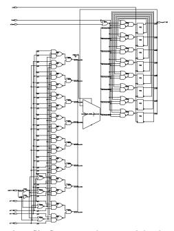
The register flip-flops are at the upper right, the adder is in the middle and the input multiplexer is at the lower left.
