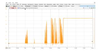
If a switch is being used in a circuit that is edgesensitive, such as the clock for a register, the signal from the switch must be "debounced" so that there is only one transition for each switch operation. This can be done by delaying recognition of changes in the switch input until the signal has been stable for a time longer than the maximum duration of the "bounces". The required duration depends on the switch, but typical maximum bounce durations would be a few milliseconds.
