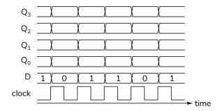
**Exercise 7:** Fill in the diagram above for a 4-bit shift register. Assume the initial value of each flip-flop is zero. Which is the oldest (first) value the D waveform? Which flip-flop holds the oldest value?
