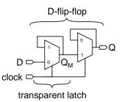
When the clock input is 0, the output of the first multiplexer follows the input – the latch is "transparent". When the clock input is 1, the output level is fed back to the input and held at that level<sup>1</sup>.
