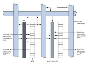
Complex software is required to fit a design into an FPGA and route the signals between logic elements. Propagation delays are harder to predict and some designs may not 'fit' into an FPGA because of insufficient routing resources.
