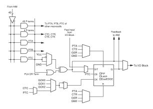
The main difference is the structure of the combinational logic – either one 4-input look-up table (LUT) per LE in for Intel CPLDs or a larger programmable logic array (PLA) driving 16 MC for Xilinx.
