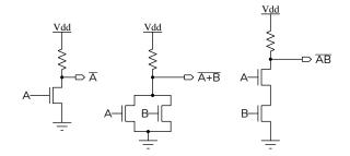
When one (for NOT), either A or B (for OR) or both A and B for (AND) inputs are high ( $>V_{th}$ ) the transistors pull the output low. The resistor (typically implemented with a transistor structure) pulls the output high otherwise.
