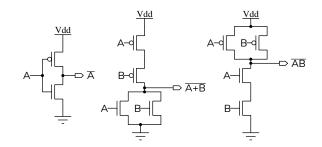
In each case the appropriate combination of NMOS transistors are turned on to pull the output low. Otherwise the PMOS transistor(s) pull the output high.
