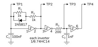
The first Schmitt trigger inverter is configured as an oscillator. When the output of the inverter is high, the capacitor charges up through a 1k resistor and the Schottky diode until it crosses the upper switching threshold  $(V_{T+})$ . Then the output switches off and discharges the capacitor through both 1k resistors in series until the input crosses the lower switching threshold  $(V_{T-})$ . The different charge and discharge rates produce an asymmetrical waveform.
