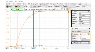
The  $\Delta$  value shown is the rise time – the time taken to go from 10% to 90% of the maximum voltage.
