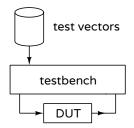
The values of the inputs and expected outputs are called "test vectors." Test vectors are often read from a file generated by other software. In this lab you will use a spreadsheet to generate a text file containing the test vectors.
