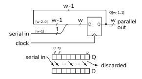
in this case the serial input bits are shifted into the w-bit shift register through the most-significant bit.
