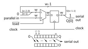
where the  $\underline{w}$ -bit register is loaded from the parallel input when  $\overline{\text{load}}$  is asserted or from the current register value shifted right by one bit. The least-significant bit of the register is the serial output.
