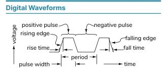
A transition from low to high is called a rising edge. The time it takes is called the rise time. A transition from high to low is called a falling edge. The time it takes is called the fall time. Two adjacent edges define a pulse, which can be negative or positive. The time between these is called the pulse width.
