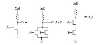
When one (for NOT), either A or B (for OR) or both A and B for (AND) inputs are high ( $>V_{th}$ ) the transistors pull the output low. The resistor (typically imple-
