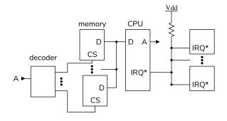
**Exercise 6:** What are the active-state current and the RC time constant for a wired-or interrupt-request line using a  $10k\Omega$  resistor pulling up a circuit with 50 pF capacitance to 3.3 V?
