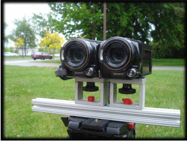
Figure 2. Stereo camera setup consisting of two identical HD camcorders.
