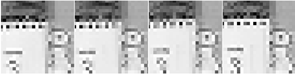
Fig. 4. Four successive frames of red Bayer pattern data, illustrating the affect of aliasing and the low correlation between frames.
