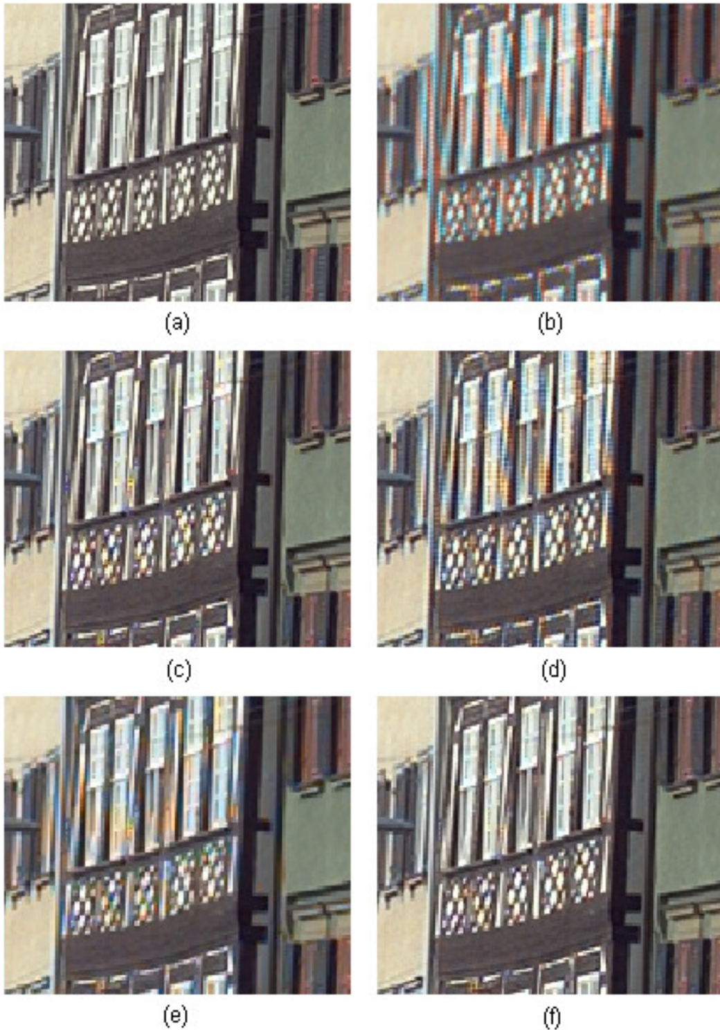
Figure 3.5: Comparison of demosaicking methods on a cropped portion of image 8. (a) original image (b) bilinear (c) method in [6] (d) method in [9] (e) YUV method in [31] (f) proposed method
