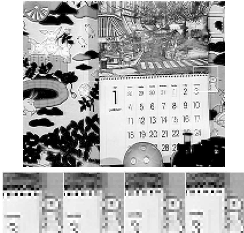
Figure 4.1: A frame of the red channel from the “Mobile and Calender” video (top), and a blowup of the highlighted region over four successive frames (bottom), illustrating the affect of aliasing and the low correlation between frames.
