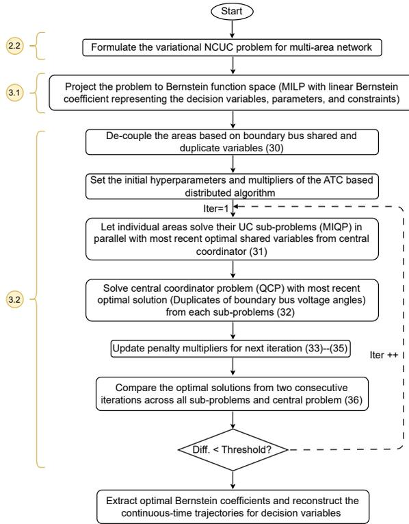
Figure 1: Flow diagram of the proposed solution methodology.
