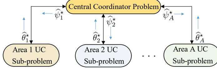
Figure 4: Hierarchical structure of an ATC algorithm where per-area UC sub-problems (31) are solved at each iteration of the algorithm and the optimal shared variables,  $\hat{\theta}^*$ ,  $a \in \mathcal{A}$ , are communicated to the central coordinator, which then solves the problem in (32) and returns the optimal duplicate variables  $\hat{\psi}^*$ ,  $a \in \mathcal{A}$ , to each area.
