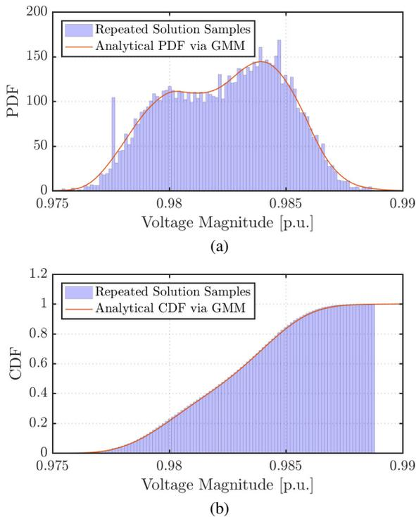
Fig. 3: Comparison of the (a) probability density/mass function and (b) probability of bus 3 voltage magnitude values obtained via (i) repeated solutions of the nonlinear power flow equations given historical EV charging data and (ii) the proposed analytical GMM-based method.
