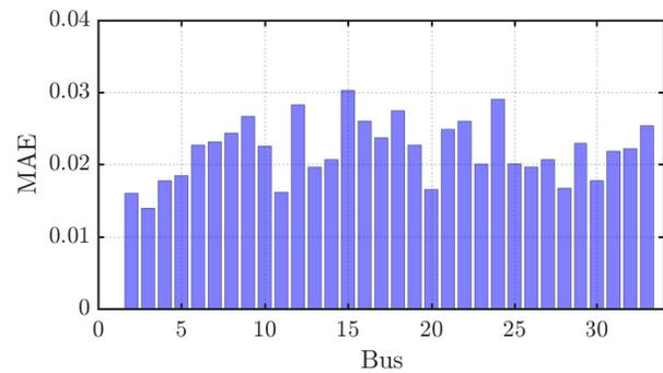
Fig. 4: MAE between repeated nonlinear solutions samples and analytical CDF via GMM for each bus.
