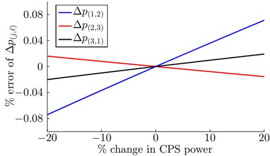
Fig. 2: Error in line flow sensitivities computed from (19) with respect to results from a numerical circuit simulation as the power injected by the CPS is varied from its nominal value of 2 W.
