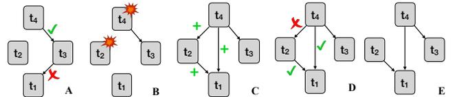
**Figure 6: Disconnected dependency recovery.** (A) dependencies are validated;  $t_3 \rightarrow t_1$  shadows the missing dependency  $t_4 \rightarrow t_1$ . (B)  $t_4$  and  $t_2$  fail because of missing dependencies. (C) recovery procedure adds candidate dependencies. (D) dependencies are validated. (E) final TDG.
