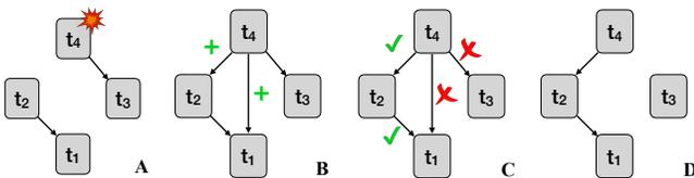
**Figure 5: Recovery of missing dependencies.** (A)  $t_4 \rightarrow t_3$  is selected,  $t_4$  fails because  $t_4 \rightarrow t_2$  is missing. (B) recovery procedure adds candidate dependencies. (C) dependency validation. (D) final TDG.
