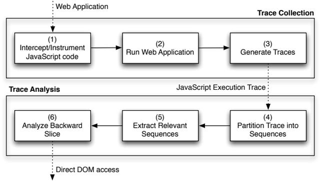
Fig. 2. Block diagram illustrating our fault localization approach.
