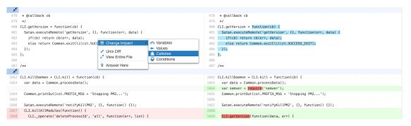
Fig. 5: A screen capture of the SEMCIA tool used in the user study. The file is sliced to show modified callsites. The slicing criterion (modified callsites) is annotated in red; dependencies (functions called by modified callsites) are annotated in blue.
