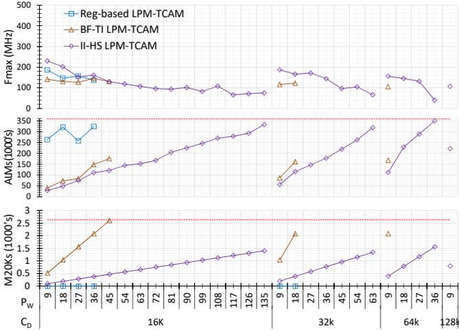
Fig. 12: Results for several TCAM depth and pattern width sweeps (bottom) M20K count (middle) ALMs count (top)  $F_{\max}$  at  $T=0^{\circ}\text{C}$ .
