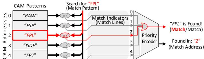
Fig. 1: CAM abstraction as a massively parallel search engine accessing all memory content to compare with the searched pattern simultaneously.
