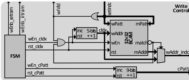
Fig. 9: Write controller, with pattern and index counters, FSM, and BCAM.
