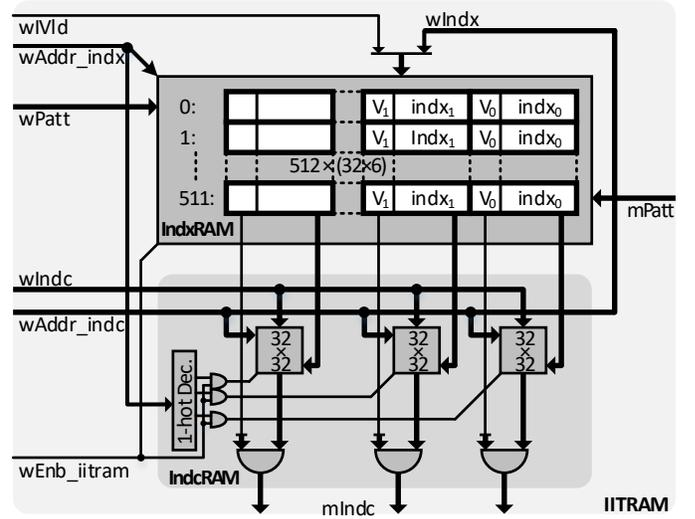
Fig. 7: Indirectly-Indexed Transposed RAM (IITRAM) unit.
