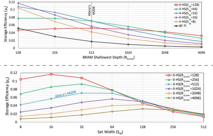
Fig. 11: Storage Efficiency  $\mu_s$  as function of (top) BRAM shallowest depth ( $d_{r,min}$ ), and (bottom) set width ( $w_s$ ) for HS-CAM and the cascaded BF.
