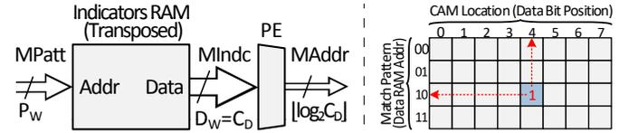
Fig. 2: (left) CAM as a Transposed-RAM. (right) Example of a pattern indicator for pattern '10' in address 4.
