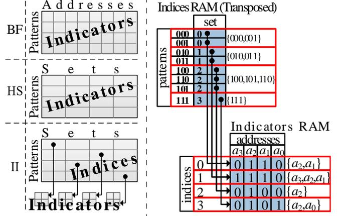
Fig. 5: (left) Indicators arrangement for three different approaches. (right) The toy example from Fig. 3, arranged as Indirectly Indexed (II) tables.
