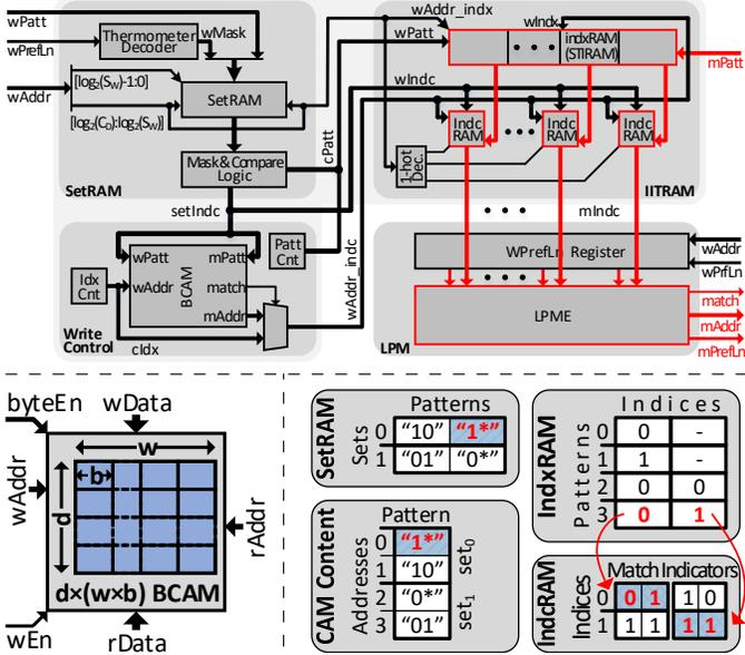
Fig. 6: (top) II-LPM-TCAM single-stage architecture. The match datapath is highlighted. (bottom-left) Dual-port block-RAM connectivity used throughout the paper. (bottom-right) Toy example of II-TCAM tables with  $d_c = 4$ ,  $w_p = 2$ ,  $w_s = 2$ . Writing "1\*" and matching "3" are highlighted.
