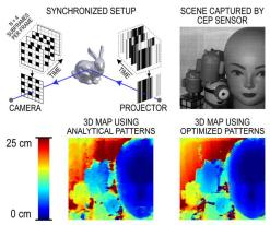
**Fig. 5:** Experimentally measured optimal structured-light 3D imaging results.
