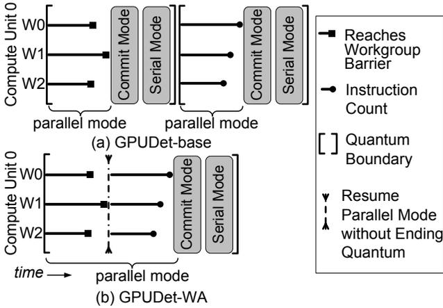
**Figure 4.** GPUdet quantum formation. (a) GPUdet-base behavior toward quantum termination events. (b) Workgroup-aware quantum formation of GPUdet (GPUdet-WA) allows wavefronts of one workgroup to continue the execution in parallel mode after all reaching workgroup barrier.
