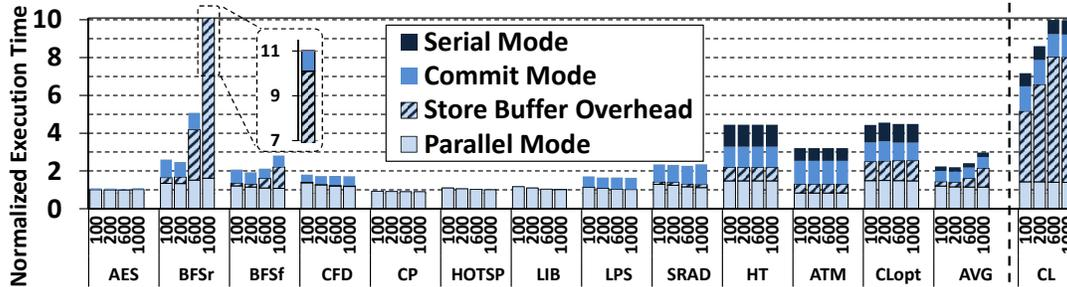
**Figure 11.** Sensitivity of GPUDet to quantum size. Execution time is normalized to NONDET. The unoptimized version of CL is not included in the average.
