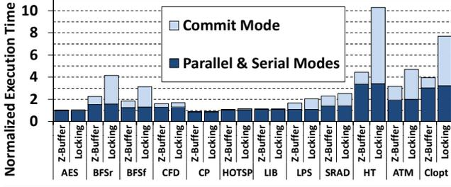
**Figure 9.** Execution time comparison of committing the store buffer between the Z-Buffer Unit parallel commit and the lock-based algorithms
