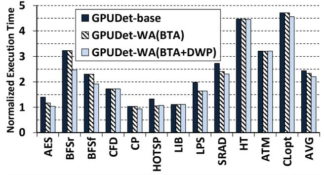
**Figure 8.** Performance impact of Barrier Termination Avoidance (BTA) and Deterministic Workgroup Partitioning (DWP) techniques. Bars Normalized to NONDET execution time.
