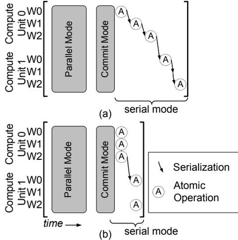
**Figure 6.** Serial mode in GPUDet. (a) Serializing execution of all atomic operations in GPUDet-base. (b) Overlapping execution time of atomic operations from each compute unit by GPUDet.
