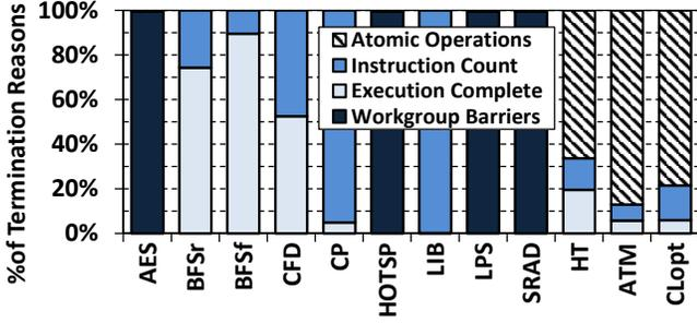
**Figure 3.** Breakdown of events that causes a wavefront to end its quantum in GPUdet with baseline quantum formation logic.
