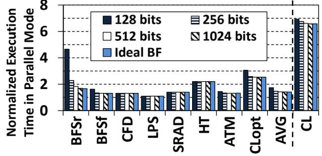
**Figure 12.** Execution cycles in parallel mode for various sizes of Bloom filter, normalized to NONDET execution. The AVG bar shows the average among all our benchmarks.
