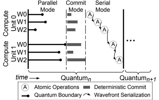
**Figure 2.** GPUDet-base architecture. Vertical lines show the global synchronization before the start of each mode. Wavefront 1 (W1) of compute unit 1 has been skipped in the serial mode since it has not reached an atomic operation in the *quantum<sub>n</sub>*.
