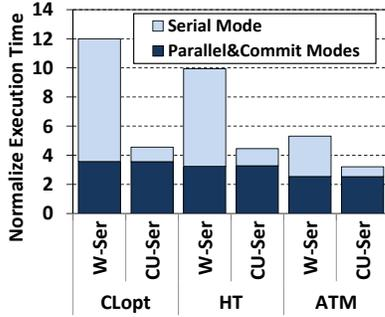
**Figure 10.** Execution time comparison between wavefront level (W-Ser) and compute unit level (CU-Ser) serialization of atomic operations (Section 4.5). Normalized to NONDET execution time
