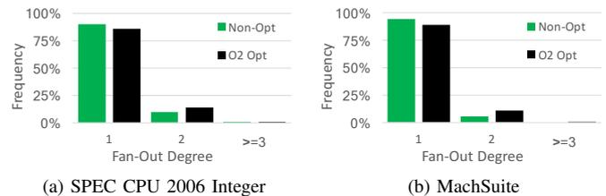
Fig. 1. Histograms showing number of successors in application *schedule flow graph* (a proxy for HLS generated FSMs using some existing HLS tools. Methodology in Section II.
