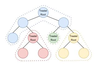
Figure 3: Example of a tree split into treelets with a maximum of 4 nodes similar to Figure 2 in [5]. Each circle represents a BVH node. Same colored nodes belong in the same treelet.
