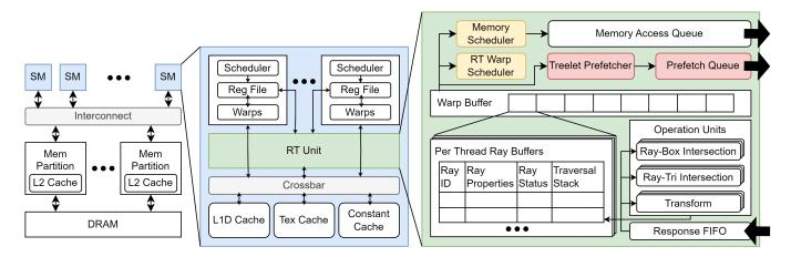
Figure 2: Baseline GPU architecture with RT Unit [41], with treelet components in red.
