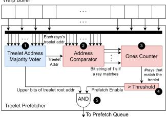
Figure 4: Hardware implementation of treelet prefetcher with treelet popularity threshold heuristic.
