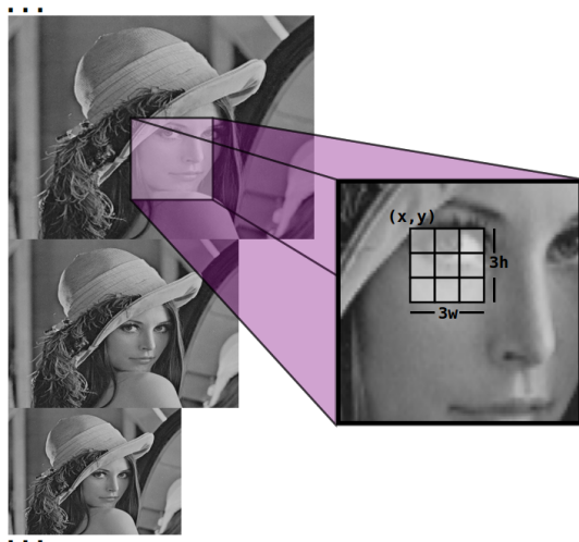
Fig. 2: Overview of MB-LBP feature detection. A search window traverses an image pyramid, and calculates multiple features at each position. Each feature compares average brightness of the center of a 3 \times 3 window against the 8 neighbours, producing an 8-bit comparison bitfield. This 8-bit LBP value produces either a PASS or FAIL value, which is summed with all features in the same stage. A stage passes, meaning a face might be present, if the sum exceeds a stage-threshold. A face may be detected only if all stages pass.
