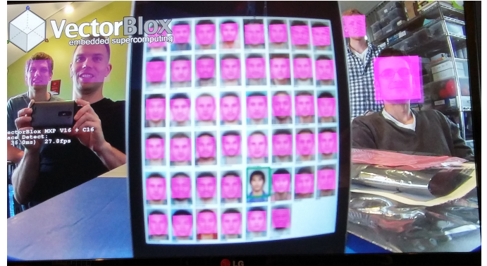
Fig. 1: Photo of video output showing 49 of 50 faces detected on a 1080p image in 36ms
