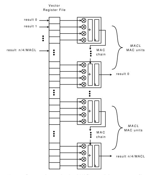
Figure 1: Connection between distributed MAC units and the vector register file
