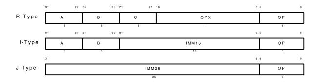
The defined vector extension uses up to three 6-bit opcodes from the unused/reserved Nios II opcode space. Each opcode is further divided into two vector instruction types using the OPX bit in the vector instruction opcode. Table 11 lists the Nios II opcodes used by the soft vector processor instructions.
