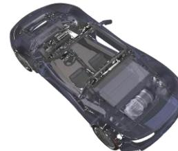
**Tesla Roadster, Induction Motor, reaches 200 kW**
