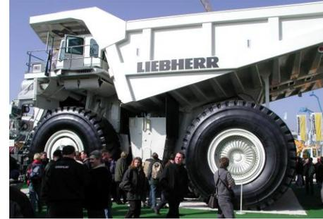
**Liebherr T282B earth-hauling truck 2.7MW AC Propulsion**
